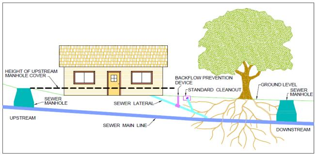
The diagram to the left depicts a typical sewer configuration. The sewer lateral carries sewage from the house to the mainline. If a blockage occurs due to root intrusion for instance, sewage will begin to backup until it reaches the lowest outlet. In this case, sewage will backup into the house before overflowing from the next upstream manhole. A backflow prevention device installed on the lateral will prevent the backup from entering the house.
