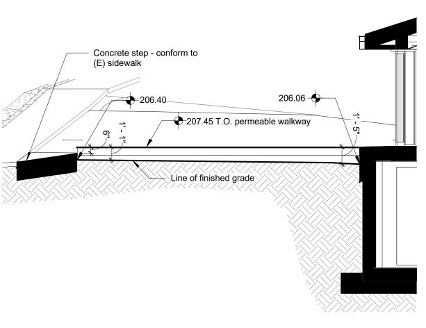
Building height shall be measured as the vertical distance from any point on the natural grade to the topmost point of the building immediately above.
