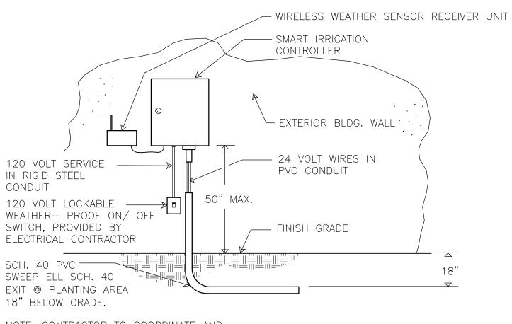
NOTE: CONTRACTOR TO COORDINATE AND INSTALL 120 VOLT POWER FROM BUILDING TO IRRIGATION CONTROLLER
