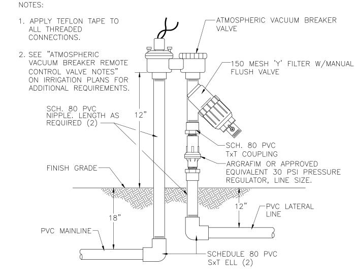
AVB REMOTE CONTROL VALVE W/ 'Y' FILTER & PRESSURE REGULATOR DETAIL NOT TO SCALE
