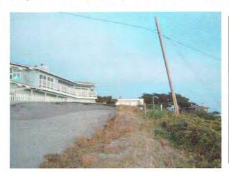
The scarp is visible as a dark wedge on the left of the photo, below the light blue house. The utility pole is one of about six that run along the west side of Ocean Blvd in this area. This is the pole that has been most affected by the movement of the slide. It is in the northern slide, near the scarp.
