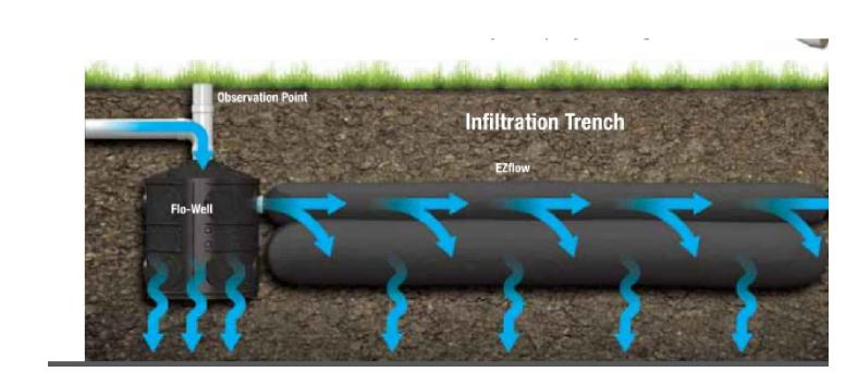
G FLOW WELL AND EZ FLOW EXTENSION SCALE: NTS
