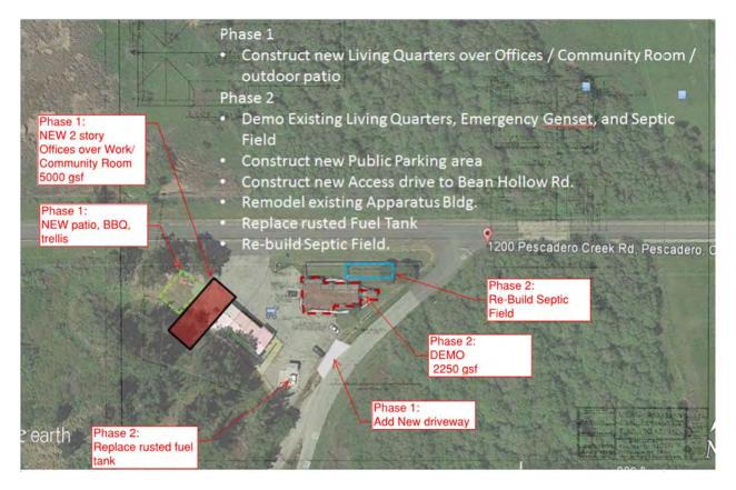
The station would consist of two separate building structures: new Office/Living Quarters and renovated Apparatus.
