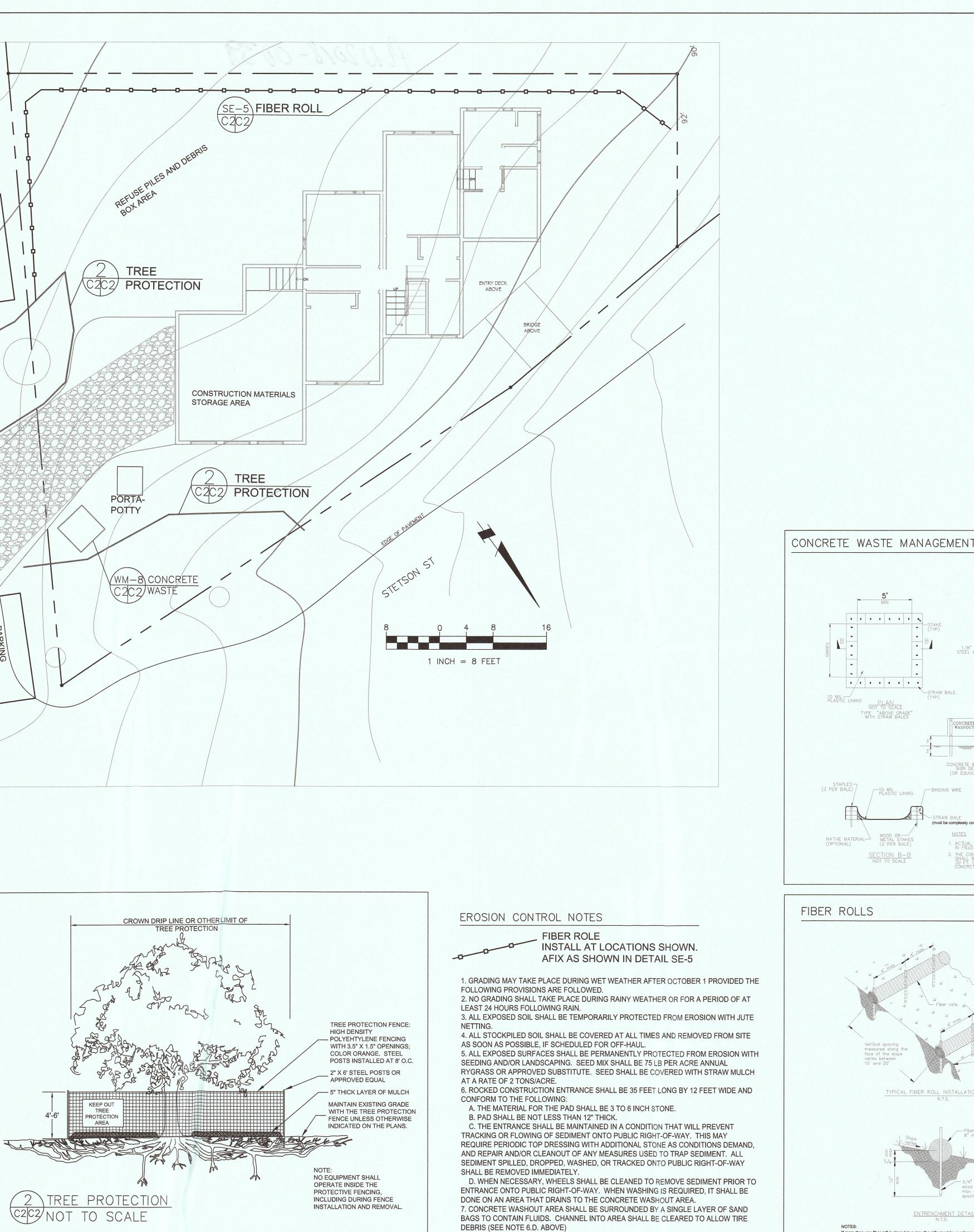
If more than one fiber roll is placed in a row, the rolls must be overlapped, not abutted Turn the ends of the fiber roll up-slope to prevent runoff from going around the roll.
