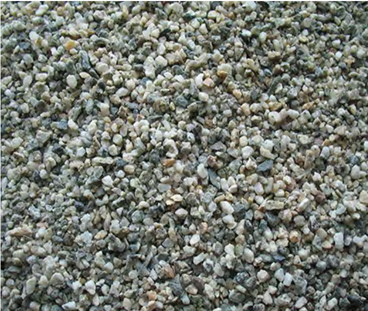
1. ROOFING: Class A 4 Ply Built up roofing finished with a layer of rock - Granite No. 4 by A1 Grit Company
