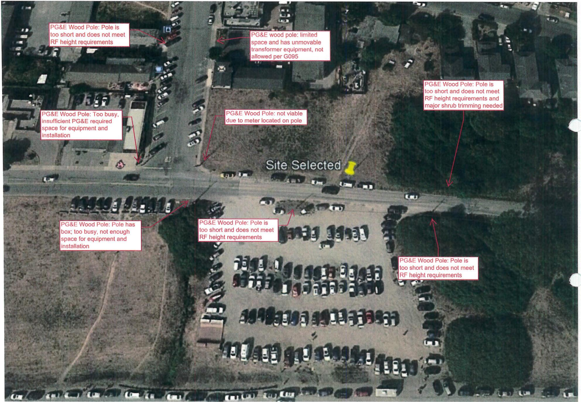
PG&E Wood Pole: Pole is too short and does not meet RF height requirements
