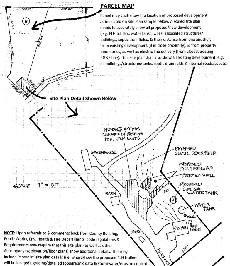
Accompanying elevation/floor plans) show additional details. This may include 'closer in' site plan details (i.e. where/how the proposed FLH trailers will be located), grading/detailed topographic data & stormwater/erosion control measures, access turn-around, new or expanded septic drain field design, additional water tanks, water line connection details, etc.
