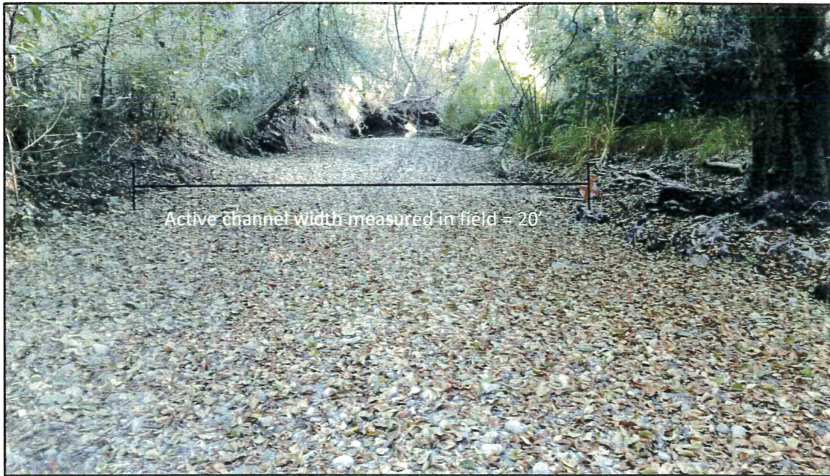
Figure A-4. Section 2, active channel width measurement, San Francisquito Creek. This section is located ~300 feet upstream of the crossing. The active channel width is 20 feet.
