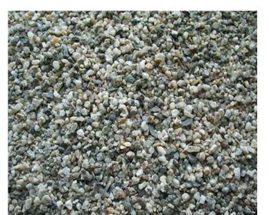
**1. ROOFING:** Class A 4 Ply Built up roofing finished with a layer of rock - Granite No. 4 by by A1 Grit
