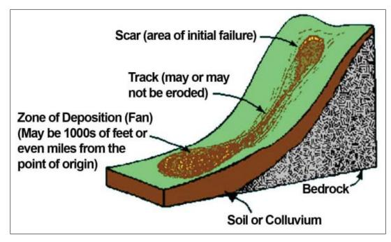
FIGURE 7-1. TYPICAL DEBRIS AVALANCHE SCAR AND TRACK
