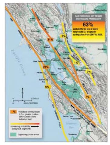
FIGURE 5-2. SIGNIFICANT KNOWN FAULTS IN THE BAY AREA
