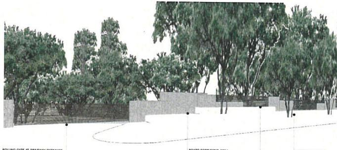
ROLLING GATE AT DRIVEWAY ENTRANCE. WOOD COMPOSITE MATERIAL BOARD-FORM CONC. WALL COMPOSITE SCRIM MATERIAL AT FENCE - 6 FT WALL MAX. (E) TREES SHOWN
