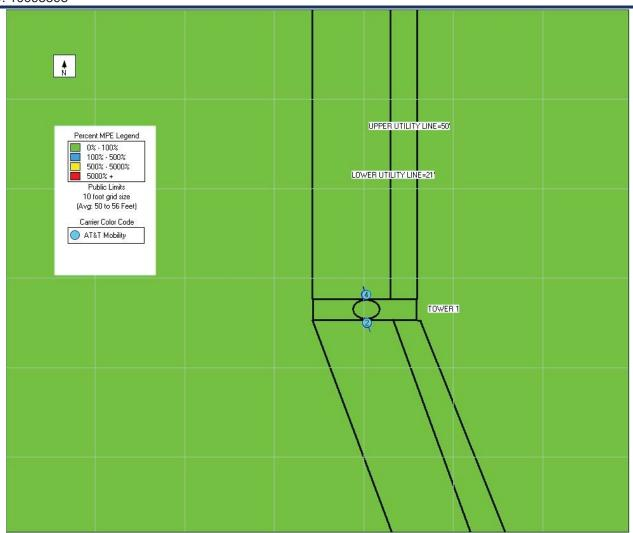
The reference plane for the plot is the 50' utility line level-Tower 1
