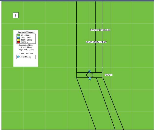
The reference plane for the plot is the 21' utility line level-Tower 1
