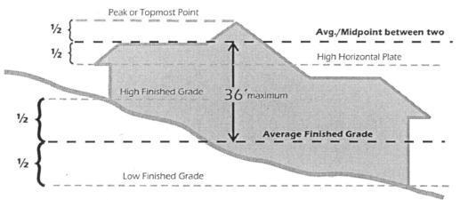
Figure 3 – Maximum Building Height Measurement
