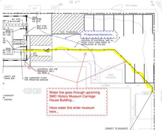
The layout of the existing domestic water line is diagrammatic because of lack of as-builts and USA field verification was inconclusive. The point of connection needs to be field verified and confirmed with Owner prior to any adjustments proposed.
