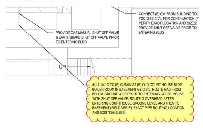
The drawing shows the diagrammatic layout of the new gas line. The path of least resistance for the actual routing of the line within the building will have to be determined in the field by the contractor. The anticipated route would be to have the gas line enter the building then hold tight to floor structure above and go into the boiler room in most direct path possible with existing conditions.
