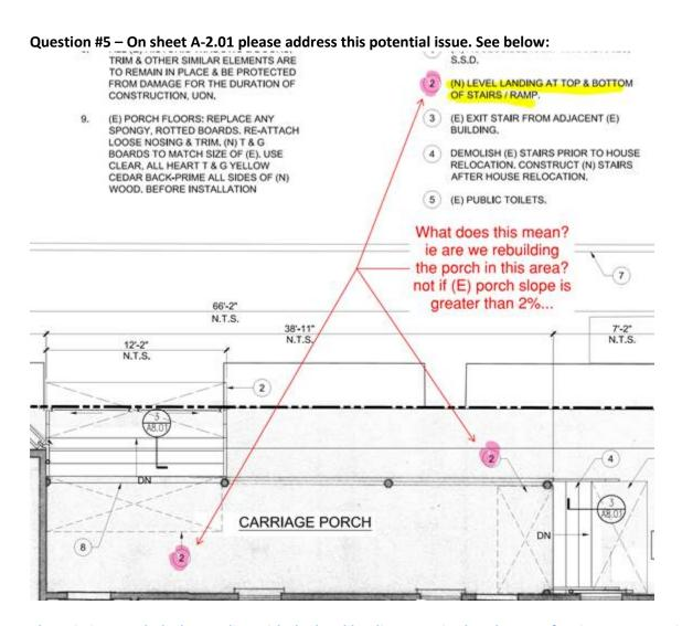
The existing porch deck complies with the level landings required at the top of stairs. Keynote 2 just clearly defines the location of the level landing which needs to remain compliant after the building relocation.
