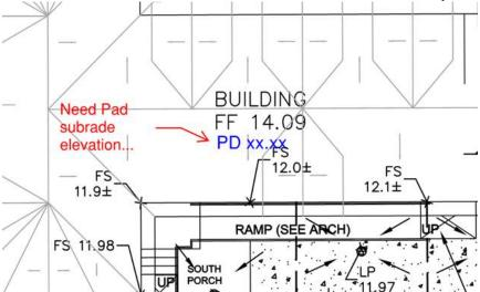
Refer to Structural plans for relationship of grade under building to finished floor. This elevation needs to be coordinated with the structural details and final code required clearance below floor joists. Determination of this elevation is outside the scope of the Civil plan set because of the potential contractor means and methods for building relocation as well as for setting the building back down onto new foundation.
