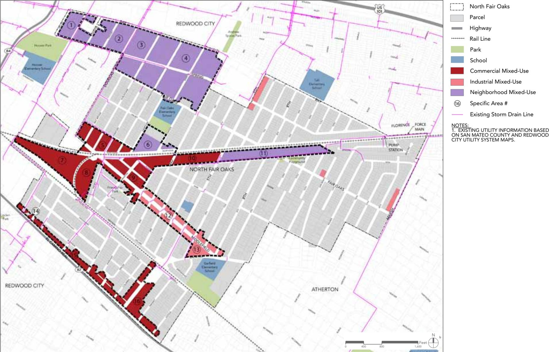
FIGURE 4.7: Proposed Storm Drain System Improvements
