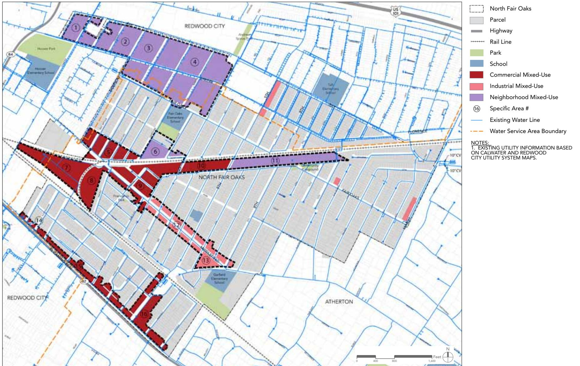
FIGURE 4.2: Proposed Potable Water System
