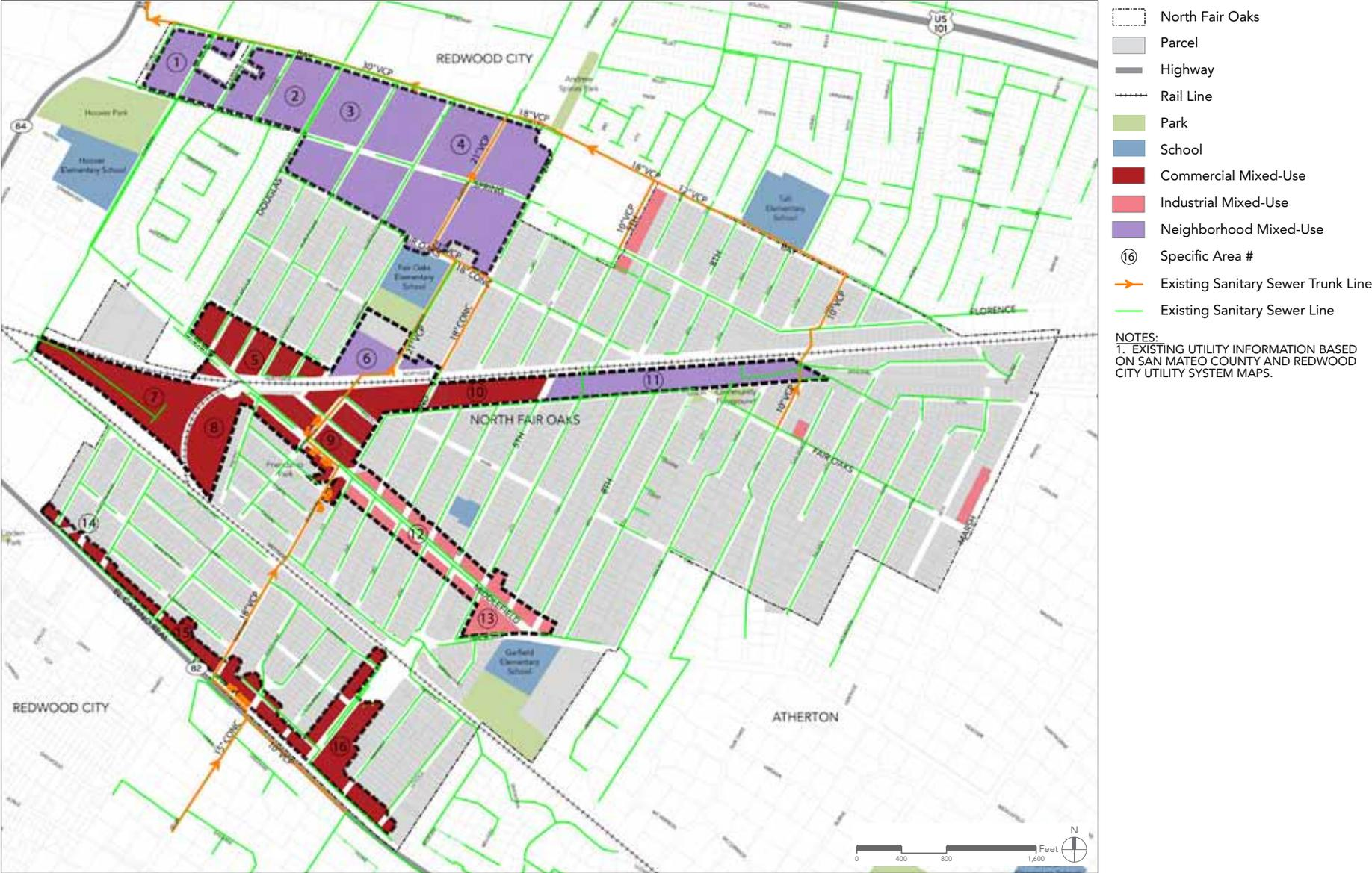
FIGURE 4.5: Proposed Sanitary Sewer System Improvements
