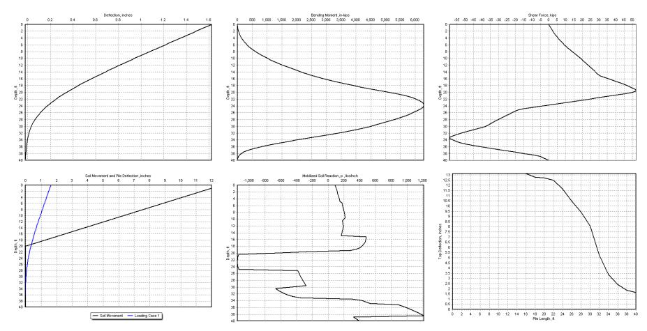
LPILE ANALYSIS OUTPUT Abutment 1, CISS = 30 x 5/8 in, Cut-off El. = 64 ft, R-17-002 With Lateral Spreading Soil Movement at Pile Top
