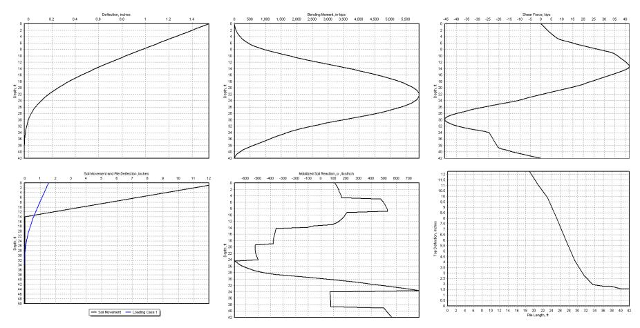
LPILE ANALYSIS OUTPUT Abutment 2, CISS = 30 x 5/8 in, Cut-off El. = 63 ft, R-17-001 With Lateral Spreading Soil Movement at Pile Top
