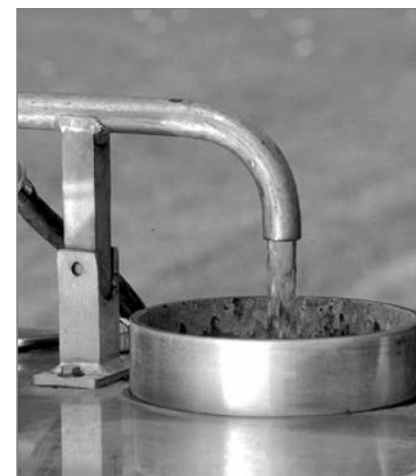
Figure 2-5. An air gap prevents back siphoning while filling a spray tank.
