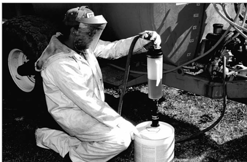
Figure 2-2. Your employees must use a closed mixing system when mixing or loading liquid formulations of pesticides with the signal word Danger .
