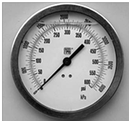
Figure 2-13. Slight changes in pressure can alter the output of your sprayer to accommodate for nozzle wear.
