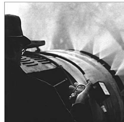
Figure 2-11. For high-pressure sprayers, spray liquid through the nozzles for a measured period of time, then measure the amount of water needed to refill the tank to its original level.
