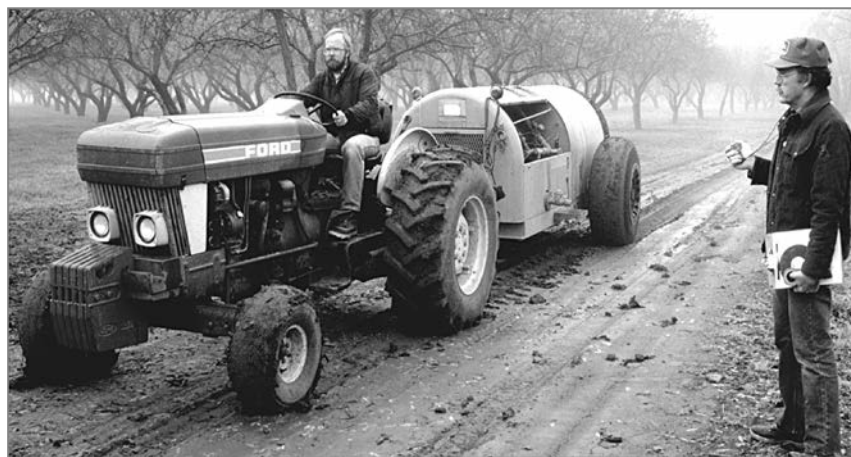
Figure 2-10. Travel speed should always be measured under actual field conditions with the spray tank half filled with water.
