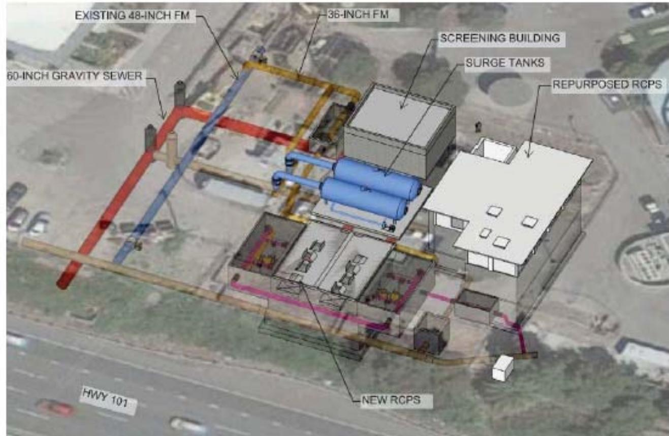
Figure ES-2. Overall RCPS layout – plan view
