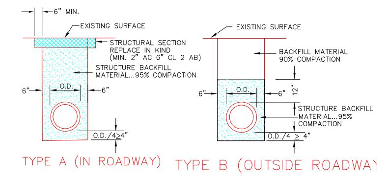
1. STRUCTURE BACKFILL MATERIAL....MATERIAL WITH SAND EQUIVALENT NOT LESS THAN 20 AND SIEVE GRADATION BY WEIGHT AS FOLLOWS:
