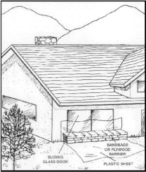
Fig.11 SLIDING GLASS DOOR SEALING
