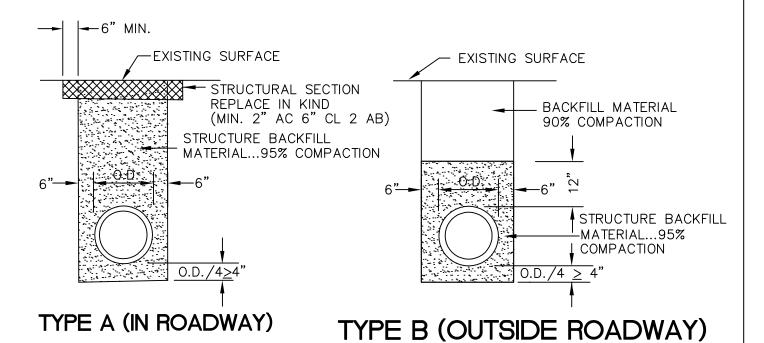
1. STRUCTURE BACKFILL MATERIAL....MATERIAL WITH SAND EQUIVALENT NOT LESS THAN 20 AND SIEVE GRADATION BY WEIGHT AS FOLLOWS:
