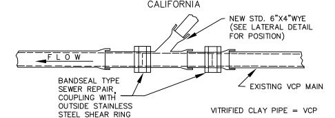
NOTE: (1) THE NEWLY INSTALLED WYE SHALL BE OF THE SAME MATERIAL AS THE EXISTING MAIN.
