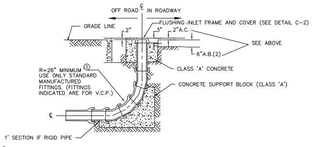
NOTE: ① FOR P.V.C. PIPE, LARGE 90° MANUFACTURED SWEEPS MAY BE USED IF R=36" OR GREATER
