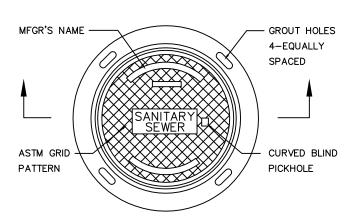
ALL MATERIALS USED SHALL CONFORM TO ASTM SPEC. A-159-70T-G3000 OR U.S. GOV'T SPEC. QQ1-653
