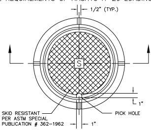
ALL MATERIALS USED SHALL CONFORM TO ASTM SPEC. A-159-64T-G3000 OR U.S. GOV'T SPEC. QQ1-653
