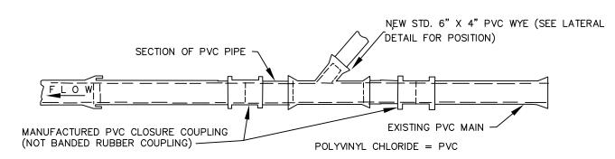
NOTE: ALL PVC, PIPE AND FITTINGS SHALL BE SDR 35 35 AND SHALL HAVE RUBBER GASKETED JOINTS. SOLVENT WELDED JOINTS SHALL NOT BE ALLOWED.
