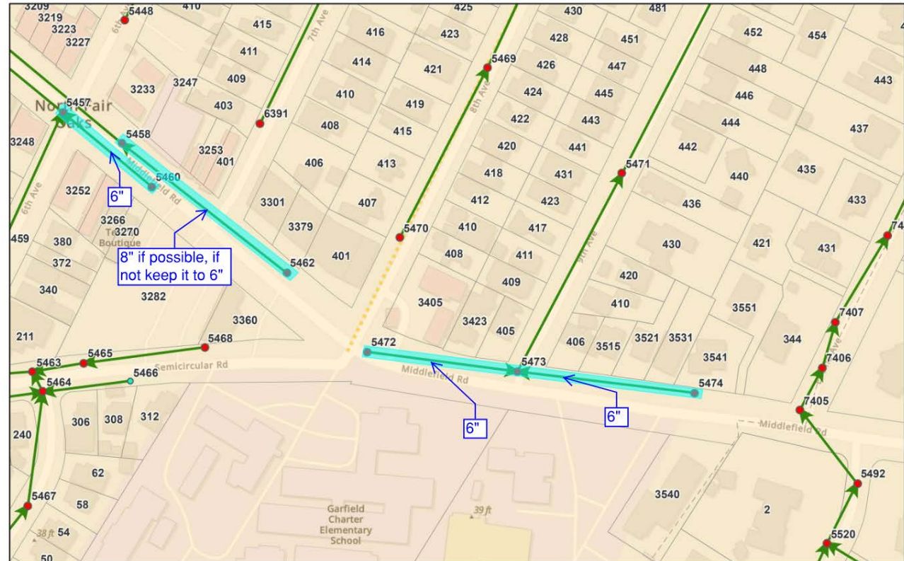
San Mateo County Sewer Facilities
