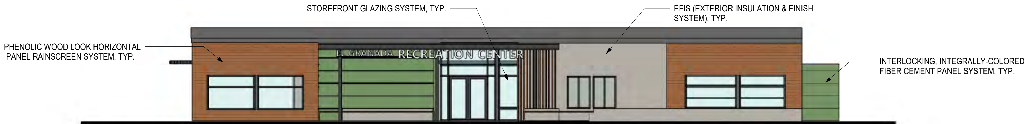
① OVERALL ELEVATION BUILDING A NORTH 1/8" = 1'-0"
