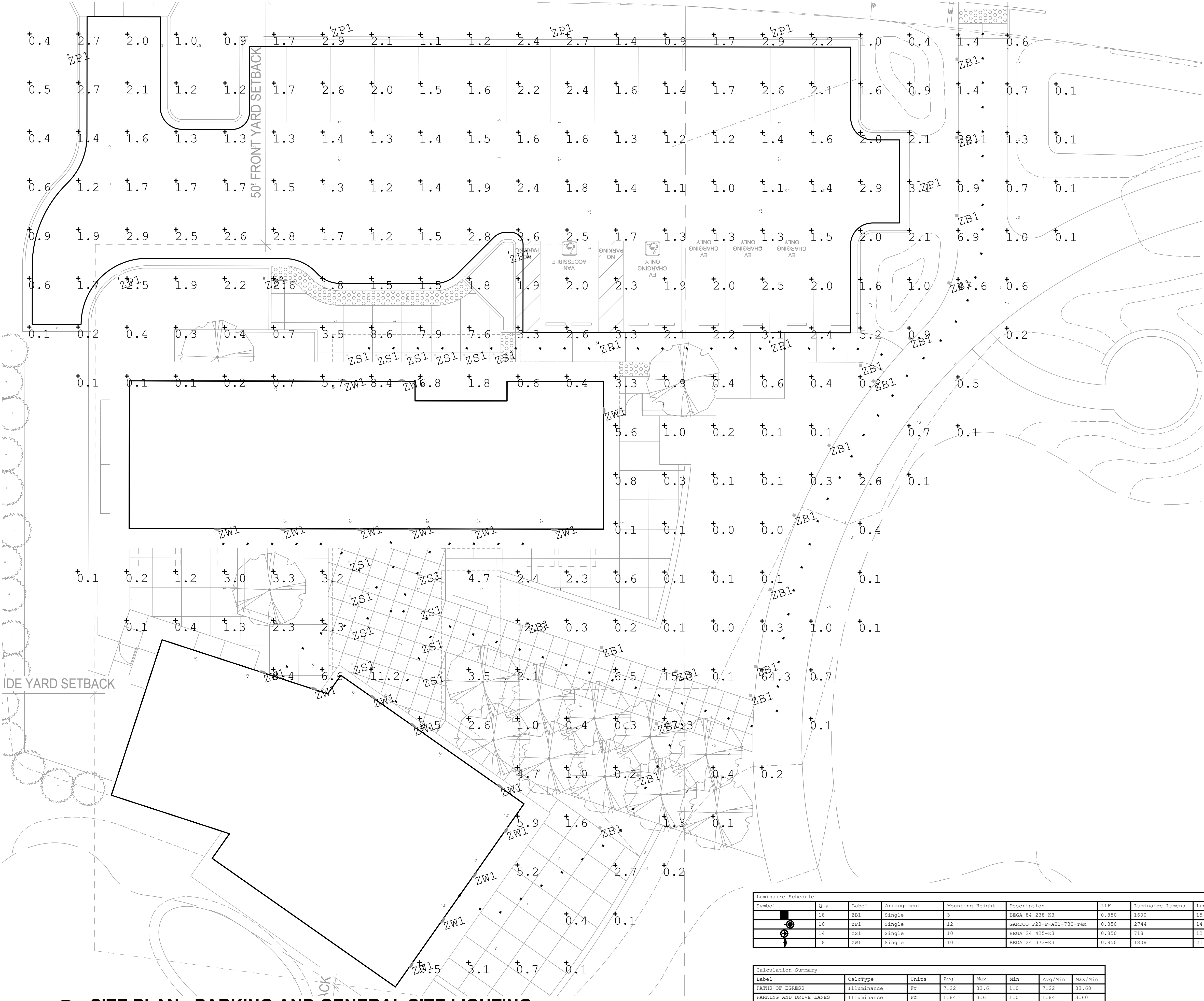
1 SITE PLAN - PARKING AND GENERAL SITE LIGHTING 1" = 10'-0"
