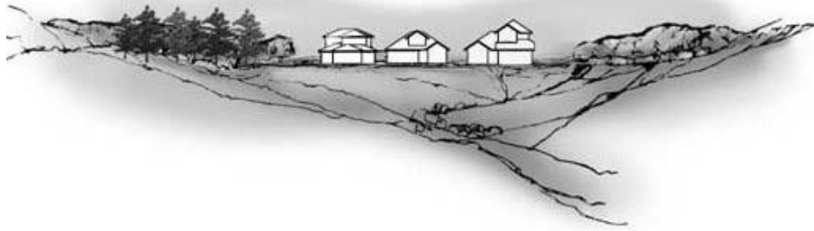
Figure 6 - In middle: Structures blend with existing landforms and vegetation. On bottom: Ridgeline silhouette has been destroyed through the removal of vegetative masses and natural landforms.
