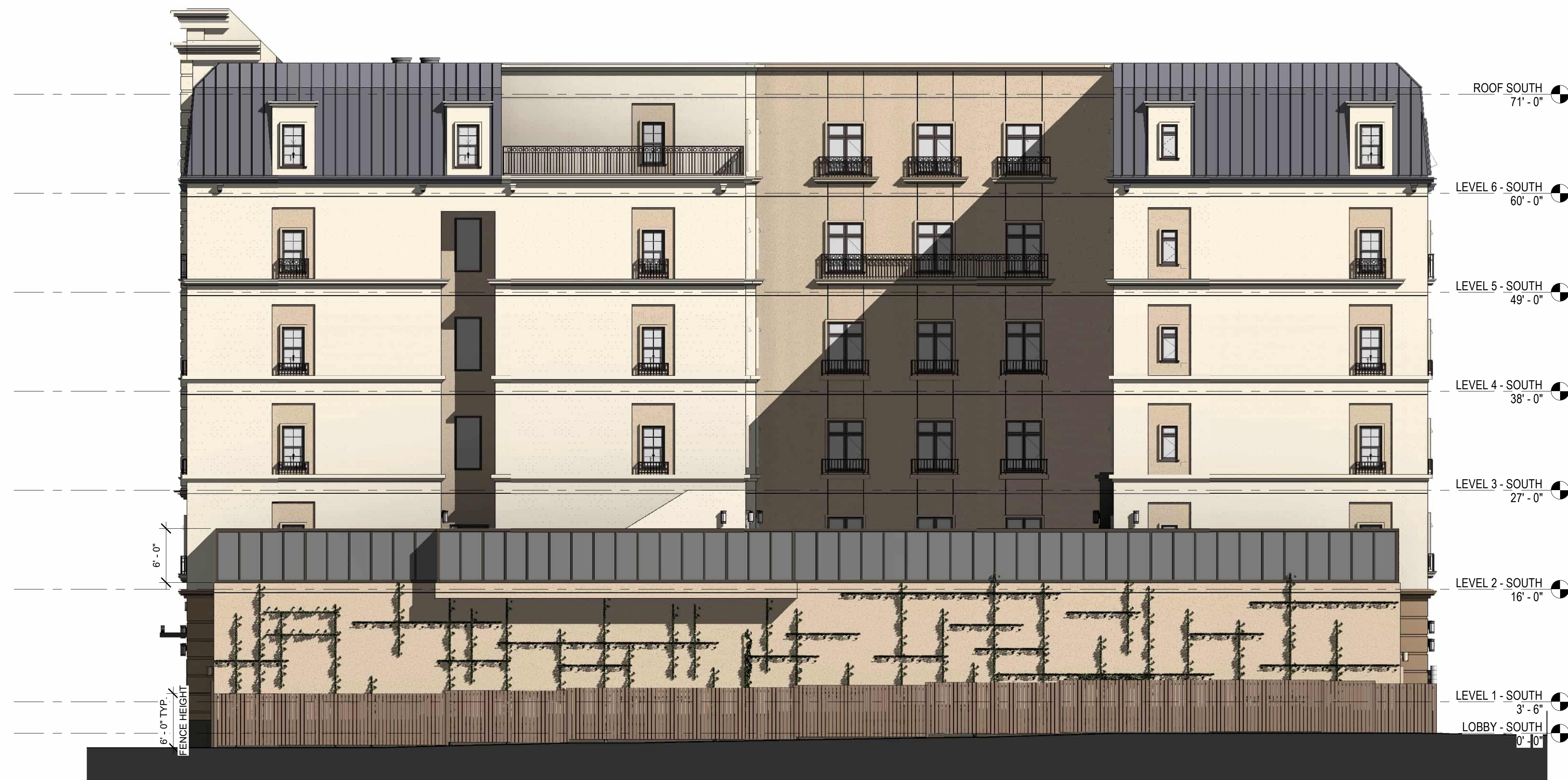
2 EAST EXTERIOR ELEVATION 1/8" = 1'-0"
