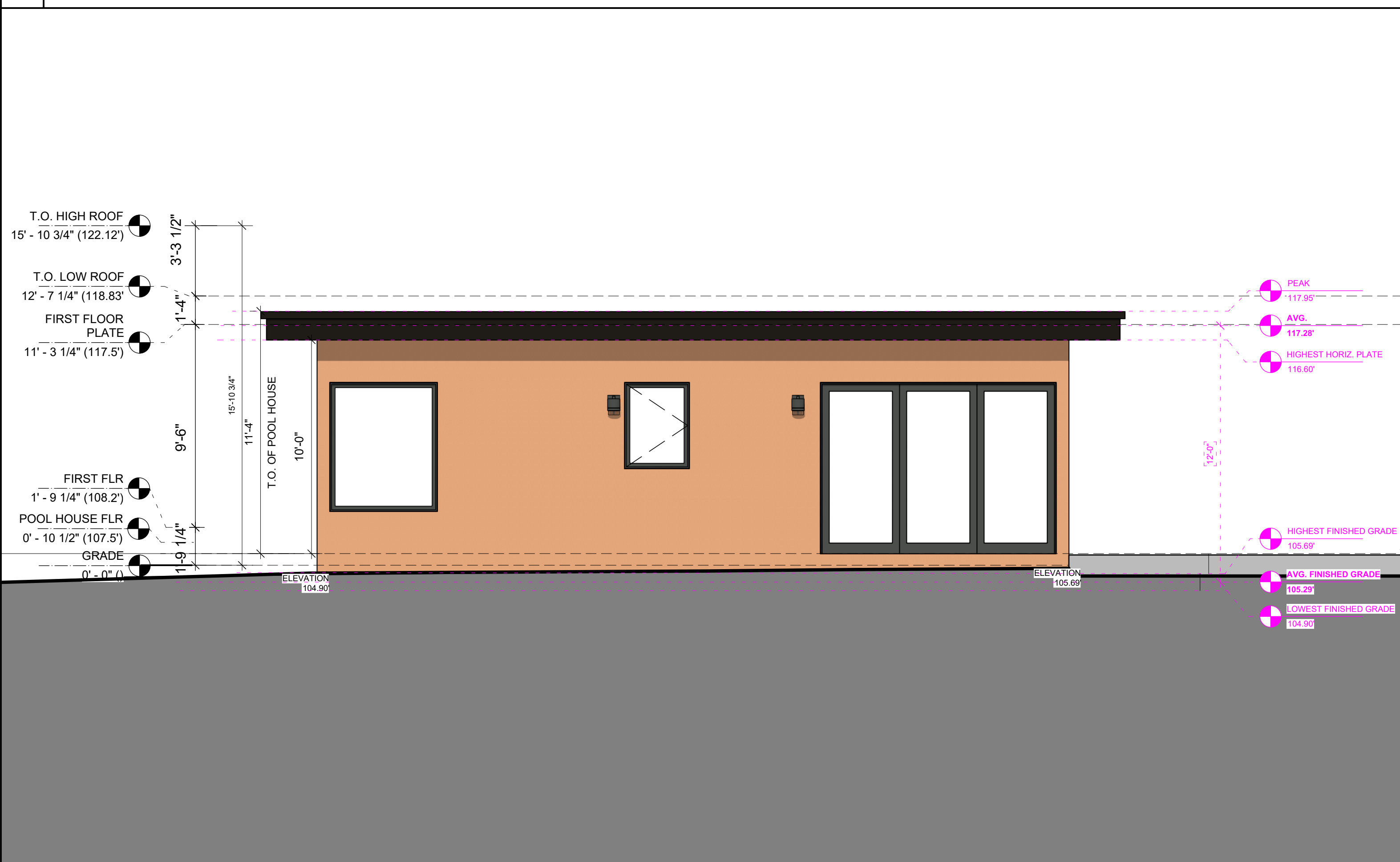
3 POOL HOUSE - SOUTH ELEVATION (FRONT) 1/4"=1'-0"
