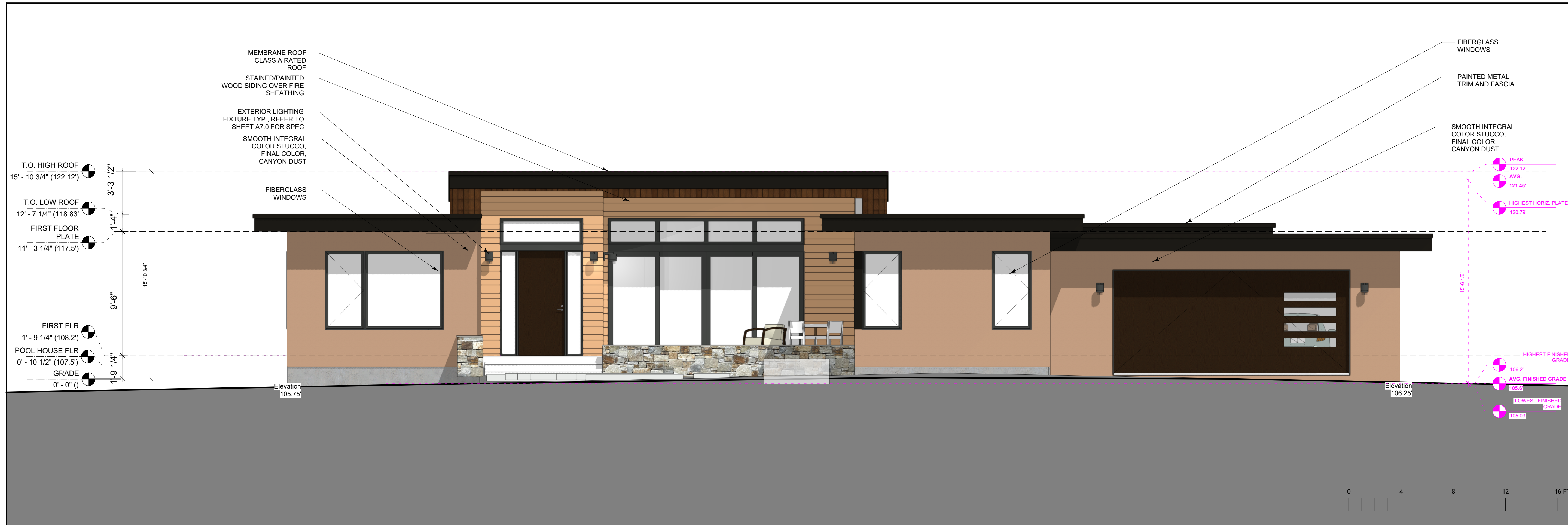
1 EAST ELEVATION (FRONT) 1/4"=1'-0"
