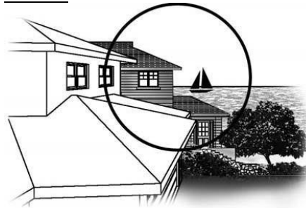
Figure 8 – on left: second story stepped back from the front and sides minimizes view blockage from neighboring homes. On right: a More massive second-story creates greater view blockage.
