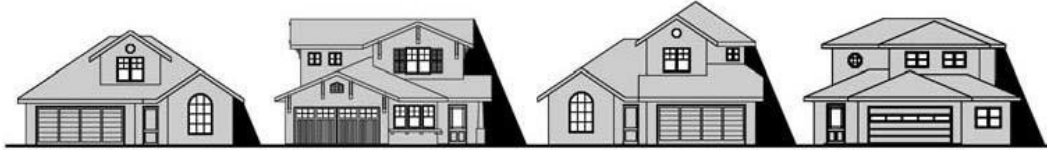
Figure 11 - These second stories held toward the center of the property allow greater sunlight into neighboring properties and help protect view and privacy.
