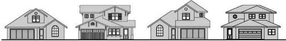
Figure 23 - These two-story houses all display roof forms compatible with their architectural style and compatible with neighboring roof forms.
