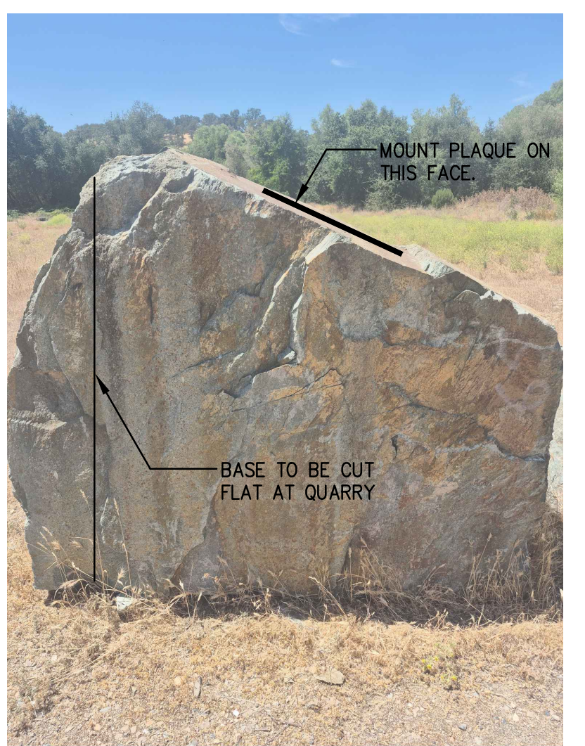
SITE 94 BOULDER BASE TO BE CUT FLAT AT QUARRY
