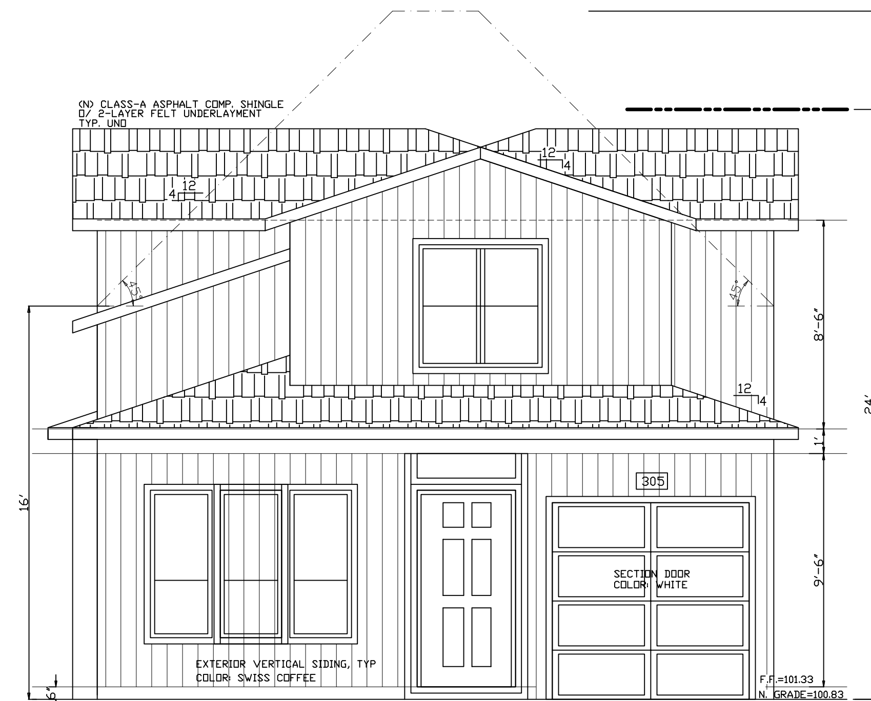
FRONT (SOUTH) ELEVATION S: 1/4" = 1' - 0"
