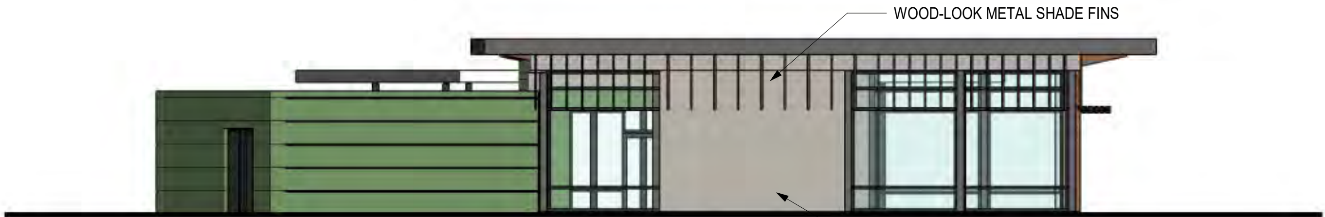
③ OVERALL ELEVATION BUILDING B NORTHWEST 1/8" = 1'-0"
