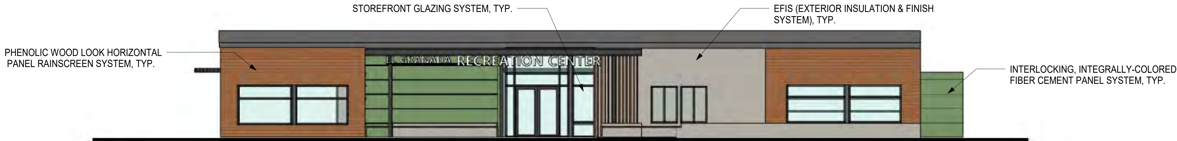
① OVERALL ELEVATION BUILDING A NORTH 1/8" = 1'-0"
