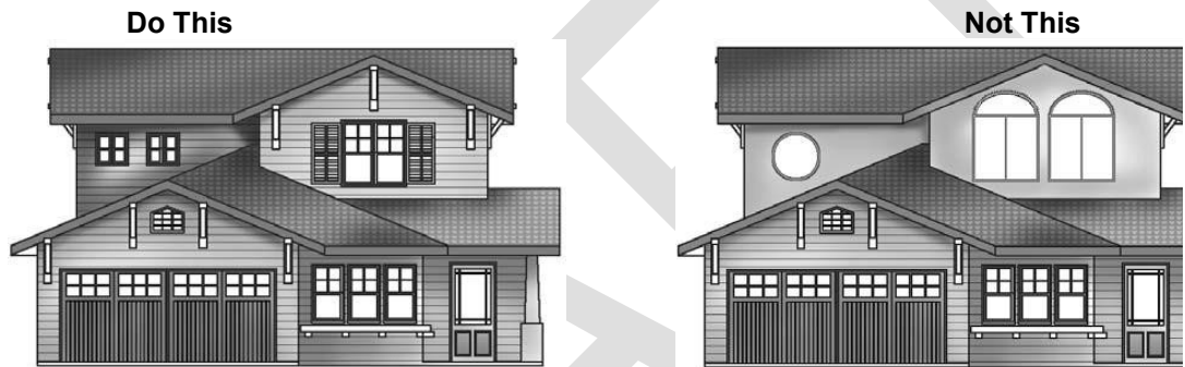
Figure 26 - On left: Style and materials of new second-story windows match and appear compatible with the original first -story of the house. On right: These new second-story windows are of different shape and proportions and material (metal vs. original wood) t
