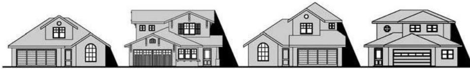
Figure 18 - These second stories held toward the center of the property allow greater sunlight into neighboring properties and help protect views and privacy.
