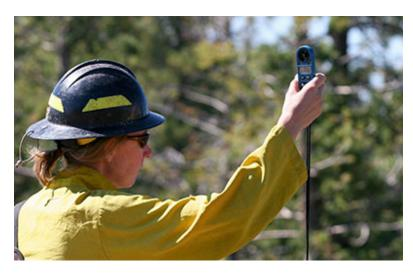
An anemometer measures wind speed. Wind is one of the factors of weather conditions that can influence wildland fire.
