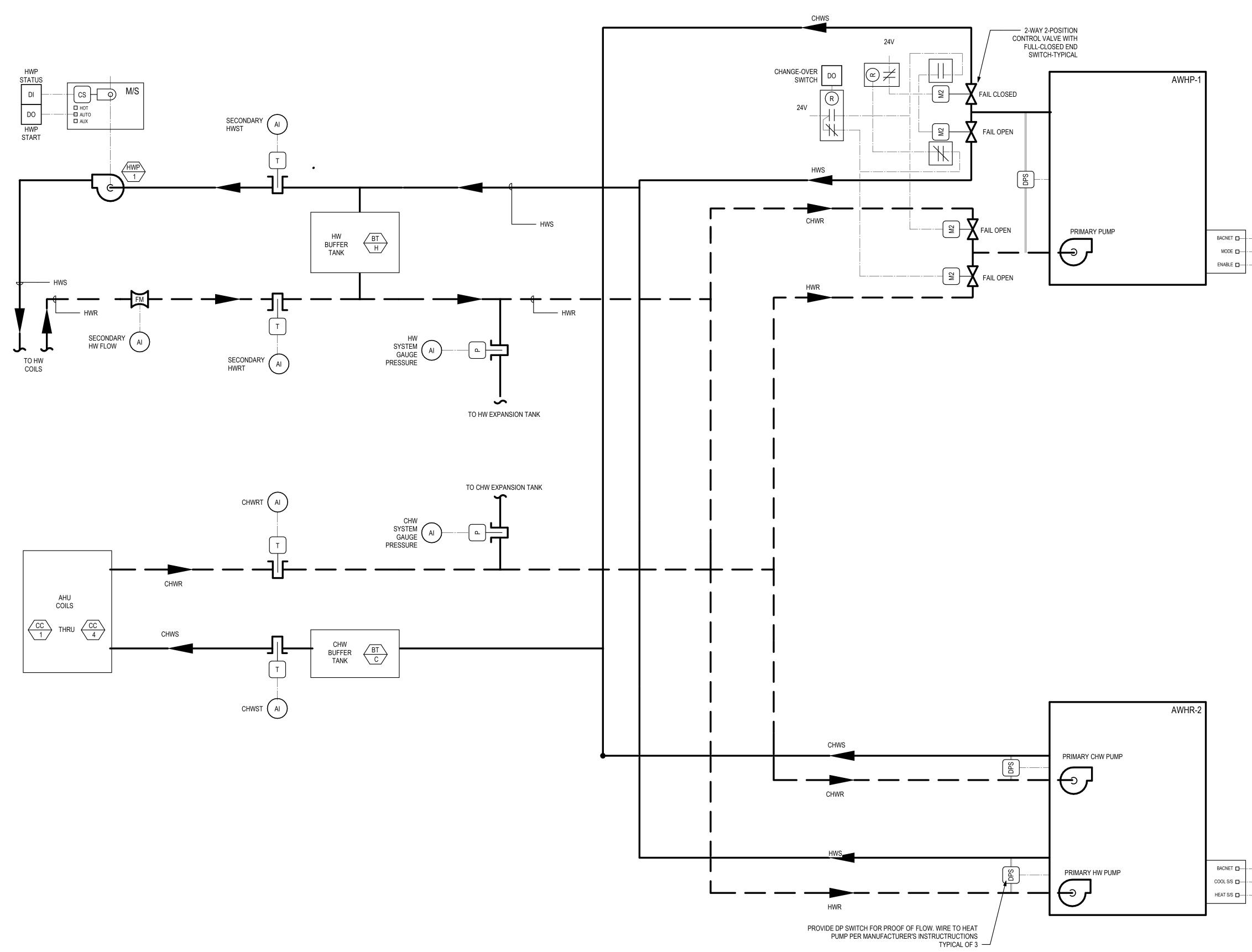
1 HEAT PUMP CENTRAL PLANT SCHEMATIC
