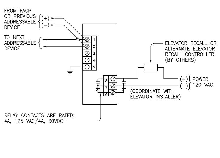
2 INTERFACE RELAY MODULE FOR ELEVATOR RECALL AND (N.T.S.) ALTERNATE RECALL FUNCTIONS
