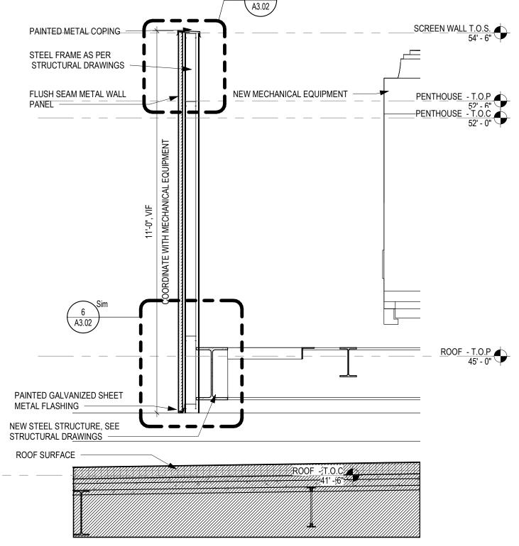
4 SECTION THROUGH MECHANICAL SCREEN
