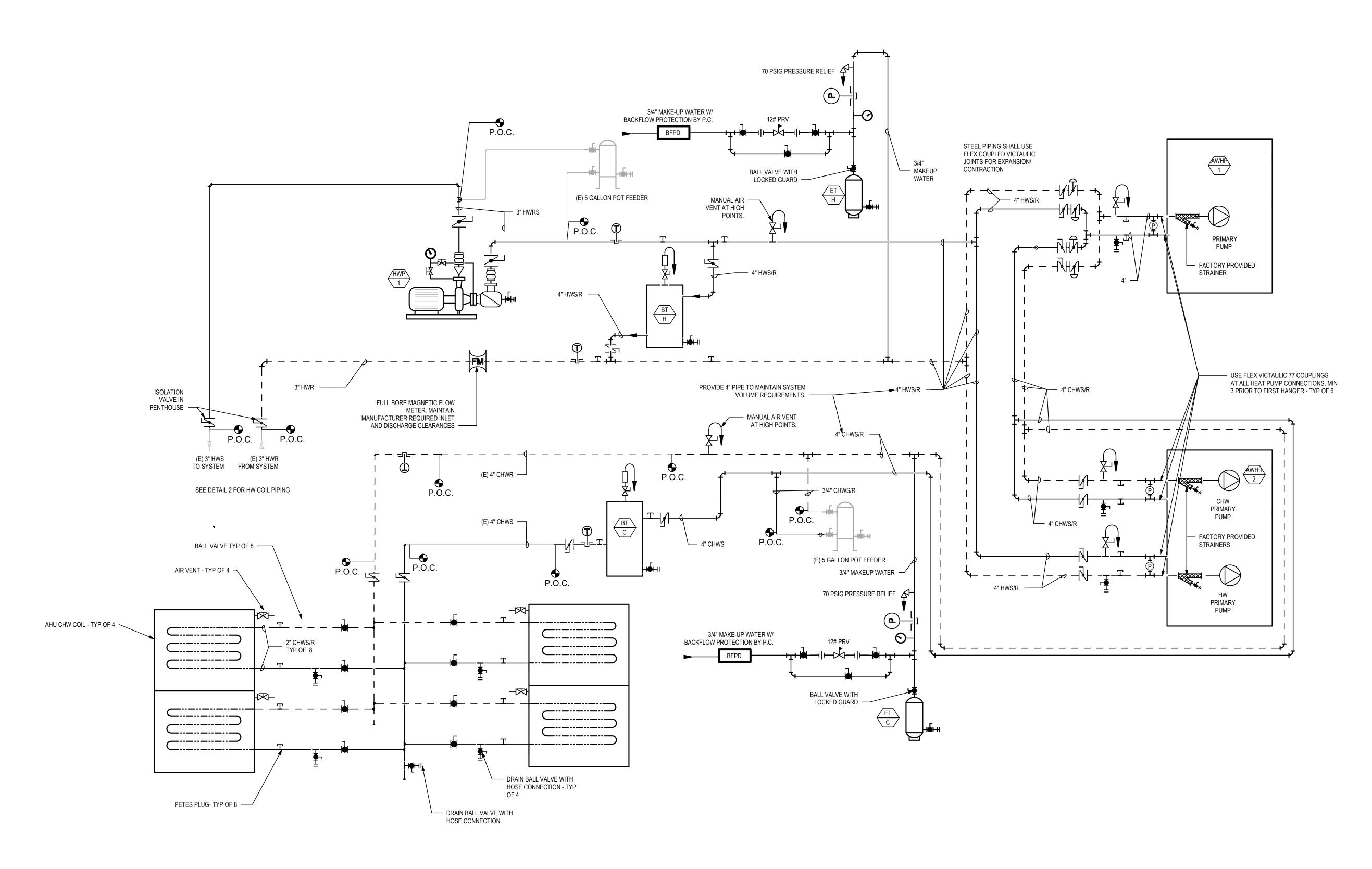
1 HW/CHW PIPING SCHEMATIC
