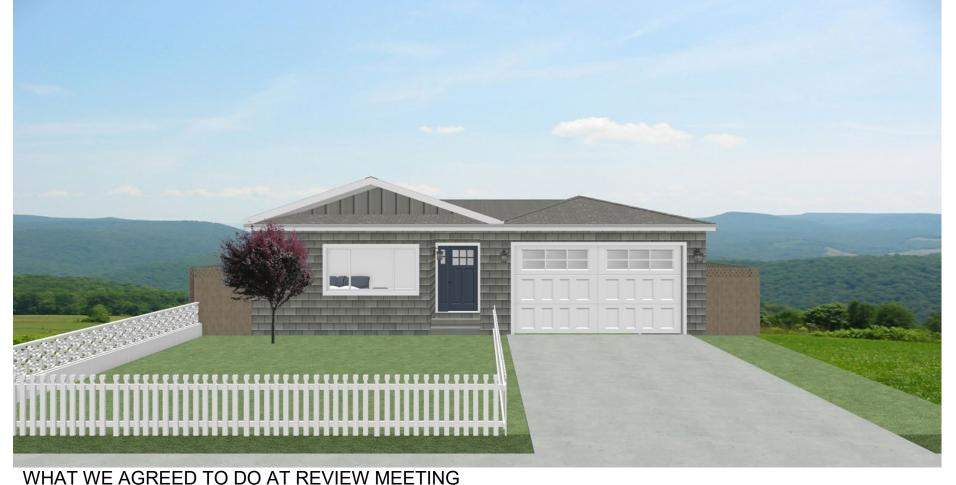
Shake siding + Board & Batten in upper areas + hip roof over garage
