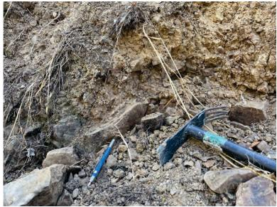
Photo 3b. Exposure at arrow in Photo 3a of closely jointed shale and graywacke mantled by Gravely Clayey Sand colluvium .
