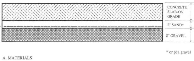
The mineral aggregate for use under floor slabs shall consist of clean rounded gravel and
