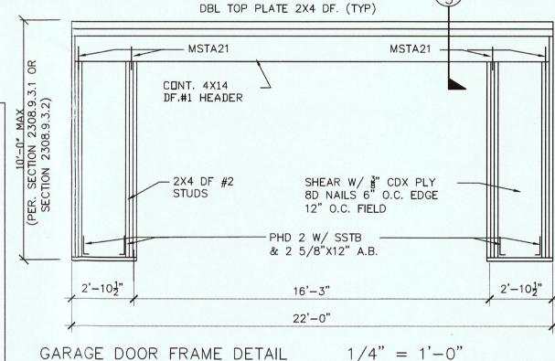
GARAGE DOOR FRAME DETAIL GABLE END (NON BEARING EXT. WALL)
