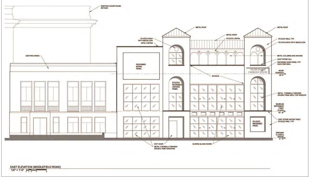
Figure 5c Building Elevations - East Elevation
