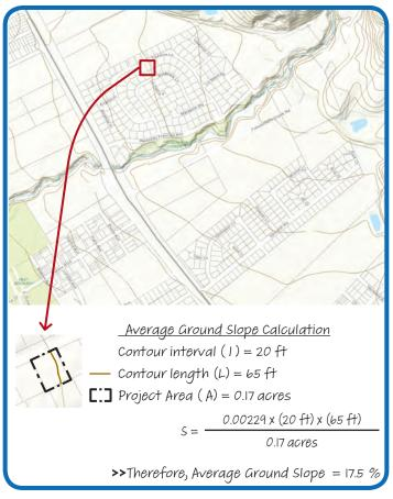
Figure 2-2. Average Ground Slope Calculation Using GIS Map Contours
