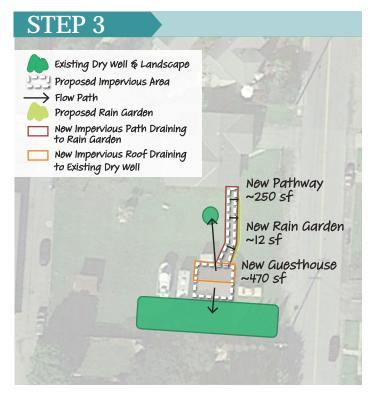
Figure 4-3. Step 3: Prescriptive Design Measure Sizing
