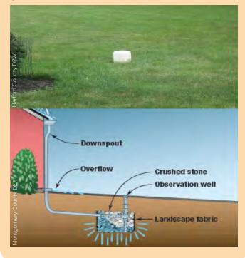
Figure 3-1. Identifying Common Drainage Facilities
