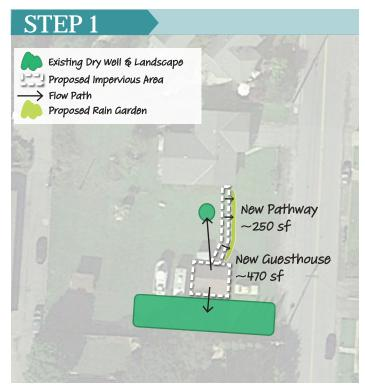
Figure 4-1. Step 1: Prescriptive Design Measure Sizing
