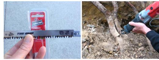
loppers, hand shears, chain saw, A/C sawzall, or other tools only under his/her direct supervision. See spec images at right. Note that a Sawzall blade indicating use for "bimetal" or "demolition" is typically not a good choice for this work. Instead, opt for a relatively large-toothed blade that indicates use for "pruning" or "wood" (see images at right).
