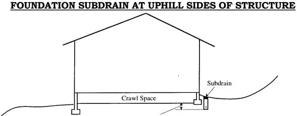
Subdrain to extend at least 6 inches below elevation of adjacent crawl space.
