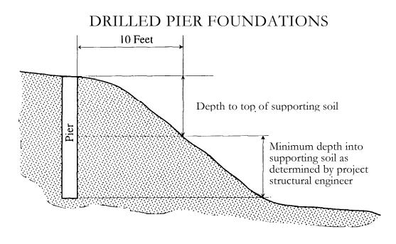
Pier depths should be based upon actual design loads at each pier location. However, as a minimum, the piers should extend 6 feet below the top of supporting material. Therefore, it is anticipated that average pier depths will be on the order of 8 to 11 feet below existing grades.
