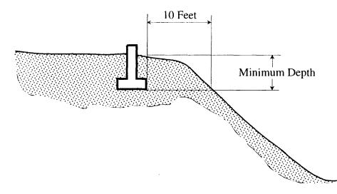
At the recommended minimum depth the footings can be designed for an allowable bearing pressure of 3000 psf for dead loads and 3250 for dead plus live loads. This value may be increased by 33 per cent to account for all loads, including wind and seismic. Page 20 December 16, 2002 Job No. 01-3186
