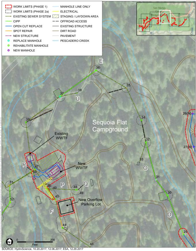
Figure 3d Phase 1 and Phase 2a Components and Work Limits
