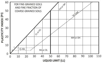
Reference: ASTM D 2487-06, Standard Classification of Soils for Engineering Purposes (Unified Soil Classification System).
