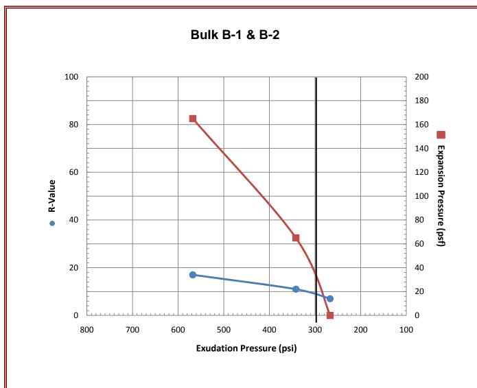
Resistance R-Value and Expansion Pressure - Cal Test 301
